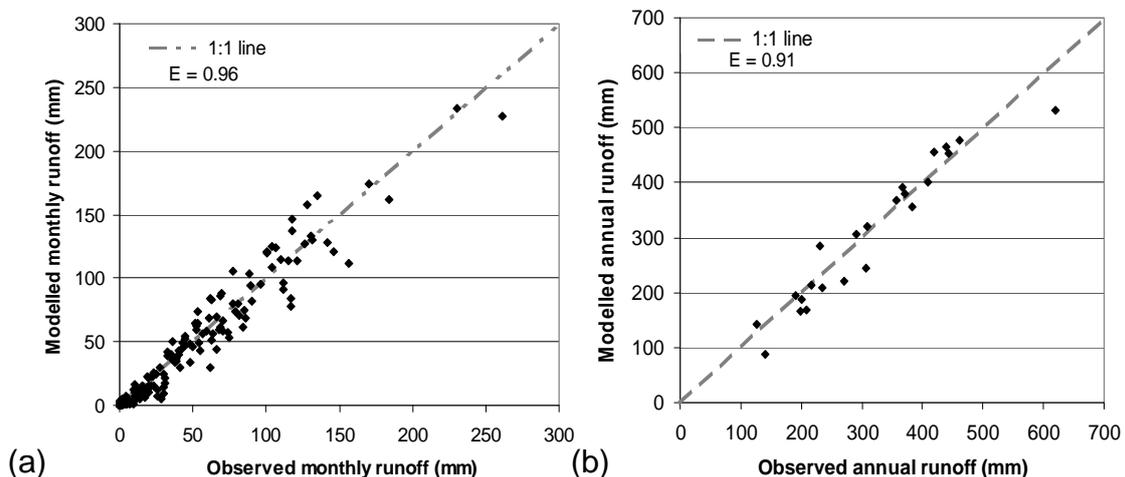
Figure 9 Modelled runoff versus observed runoff at Woodlands gauge: results for (a) monthly timescale and (b) annual timescale
