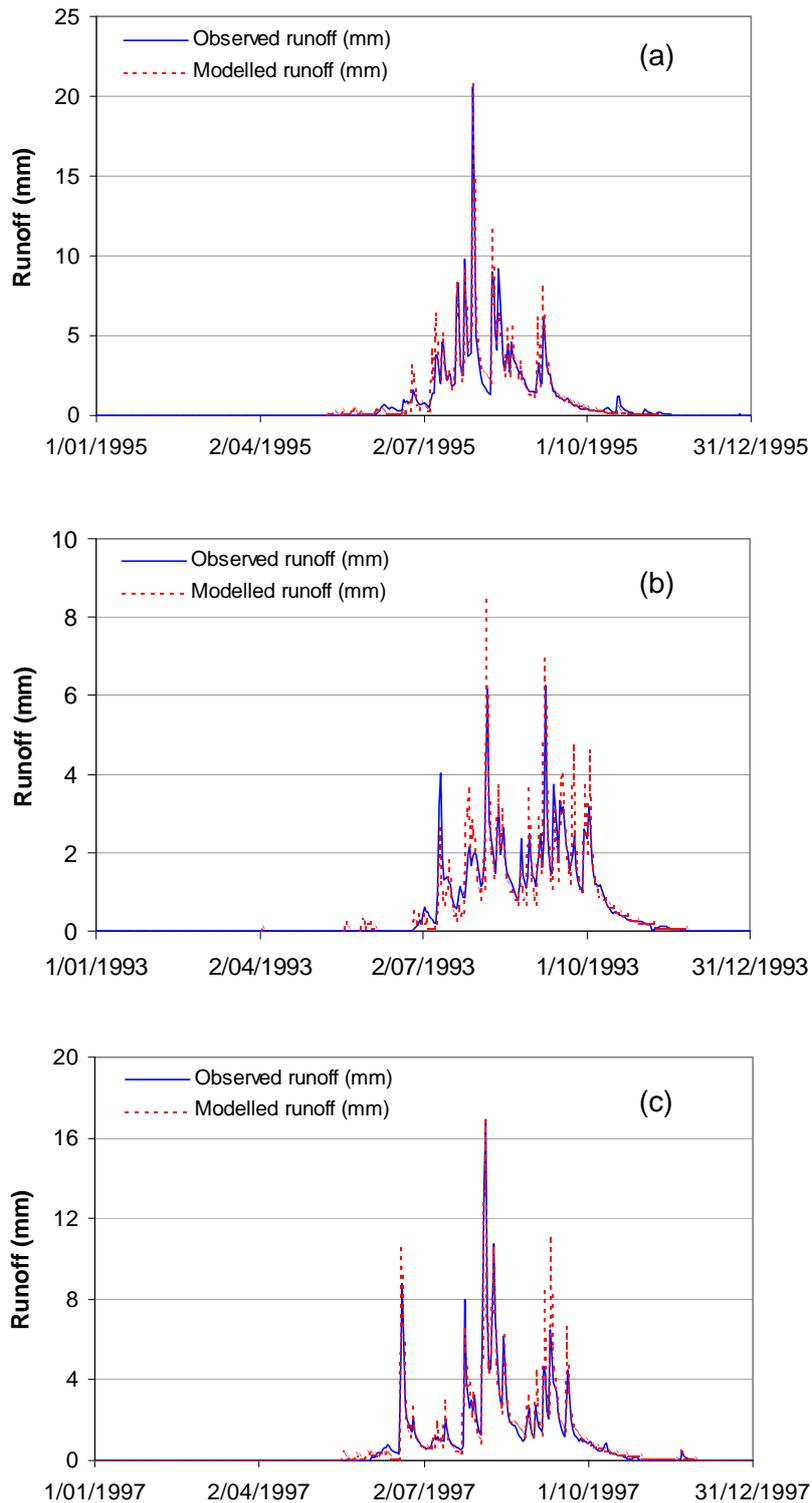
Figure 10 Comparison of observed and CSS-modelled daily flows for (a) a calibration period average-flow year (1995), (b) a calibration period low-flow year (1993) and (c) a verification period average-flow year (1997)
