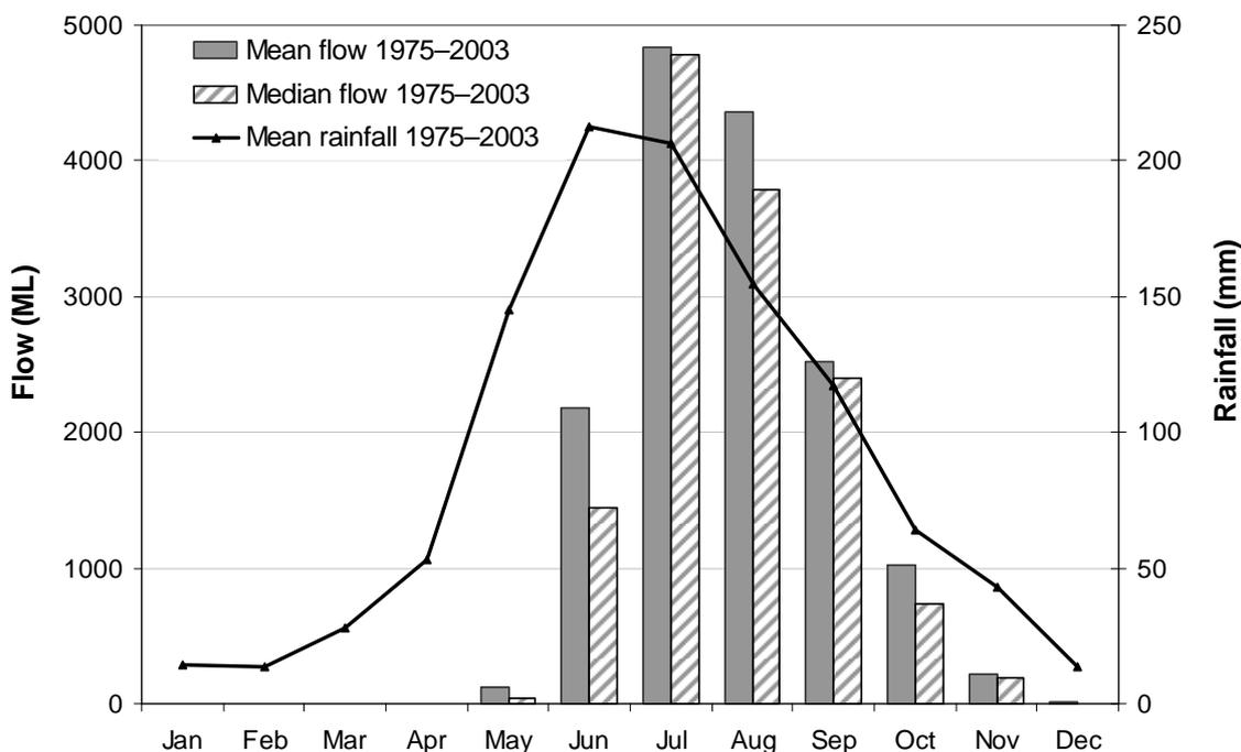
Figure 22 Mean and median streamflows at Juniper and mean rainfall at station 009636
