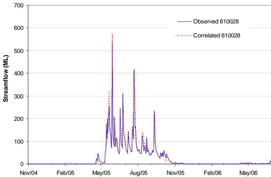
Figure 20 Verification of the compatibility of the transformed data series to the observed record at Juniper - 610028
